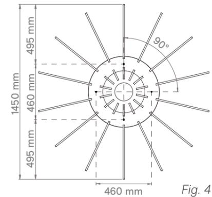
Determine where you want the Lattice to hang (Fig. 4). Mark the ceiling fixing points as per dotted lines.
