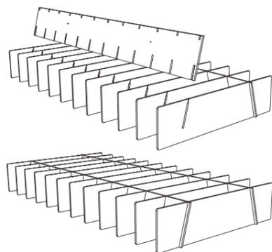
Once all the fins are inserted into the rail, flip the Lattice over 180°. Slide the remaining rail into the slots on the fins; again ensuring the tabs on the fins click into the groove on the rail.
