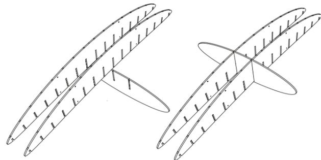
Sort the Lattice 'fins' into pairs, then into size order: largest to smallest. Start by taking one of the largest fins and slotting it into the centre slots in the 'rails'.
