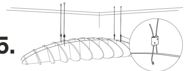
Lift the Lattice up to meet the cables threading the wires through the plugs and into the cable adjuster.
