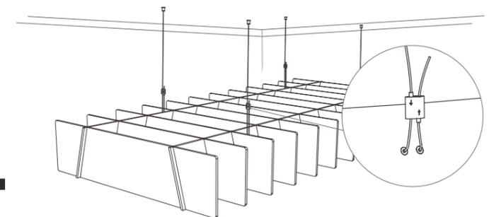
Lift the Lattice up to meet the cables and thread the wires through the plugs and into the cable adjuster.
