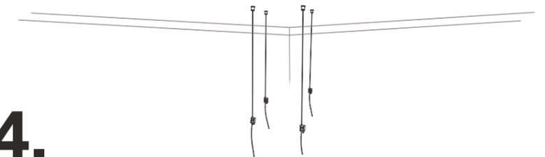
Screw assembled cables into the fixed ceiling mounts.
