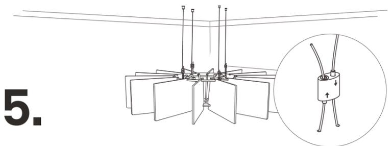
Lift the Lattice up to meet the cables, thread the wires through the holes in the top ring and insert into the cable adjuster.
