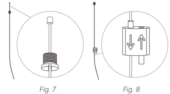
Thread the ceiling mount caps (Fig. 6) onto the cables (Fig. 7).
