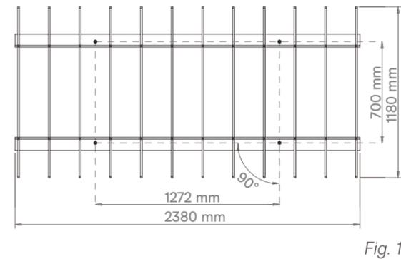
Determine where you want the Lattice to hang (Fig.1). Mark the ceiling mount points as per the above diagram.
