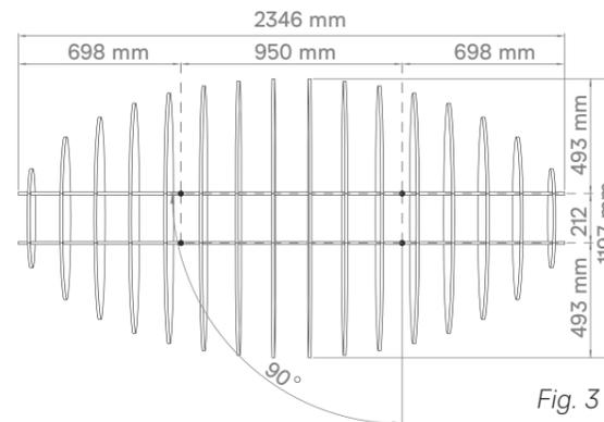
Determine where you want the Lattice to hang (Fig. 3). Mark the ceiling mount points as per the dotted lines.
