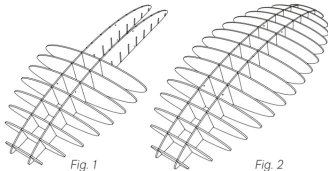
Finish one side by methodically inserting one of each pair into place in order of decreasing size (Fig. 1).
