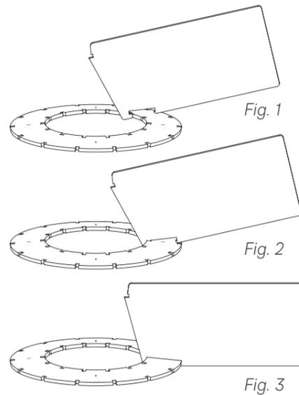
Start clipping the fins into the top ring as shown in Fig. 1, 2 and 3 until complete.
