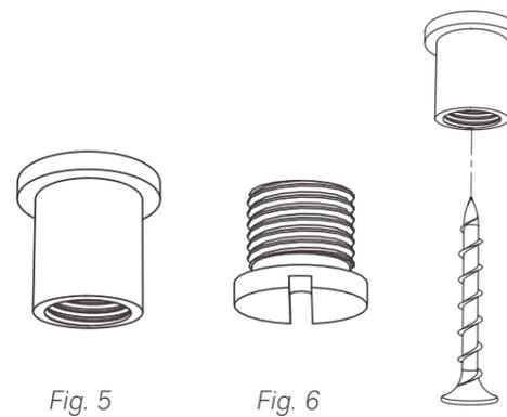
Separate the ceiling mounts into their individual parts - ceiling mounts (Fig. 5) and ceiling mount caps (Fig. 6).
