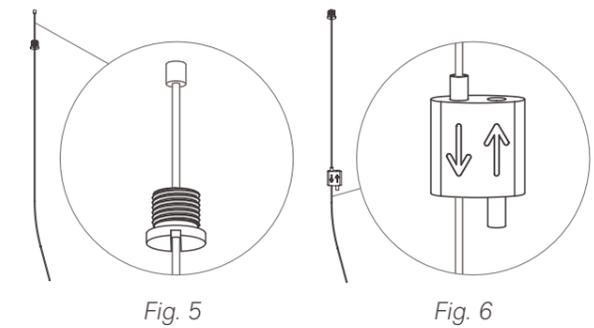
Thread the ceiling mount caps (Fig. 4) onto the cables (Fig. 5).
