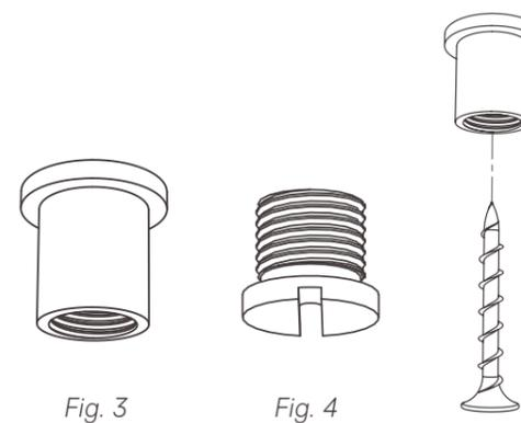
Separate the ceiling mounts into their individual parts - ceiling mounts (Fig. 3) and ceiling mount caps (Fig. 4).
