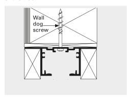
Care must be taken not to contaminate the inside of the track or to use the incorrect screws.
