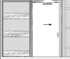
c) Open the door again and loosen the activator grub screws.
