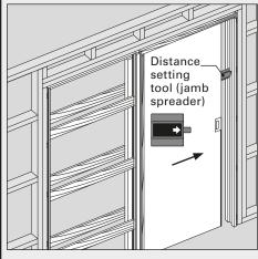
e) Without moving the activator, open the door and securely tighten all four grub screws.
