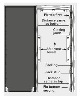
13. AluSealed units: Screw through predrilled holes in the centre of the closing jamb. Aluminium plugs are supplied to cover the fixing holes. Put these in only when you are satisfied with the complete installation!
