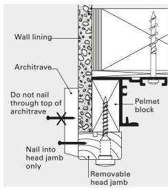
AluSealed: When fixing wall linings above the head jambs do not allow the linings to finish lower than 5mm below the top of the head jamb.
