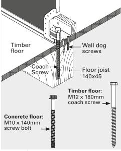
Drill 2x Ø9mm holes at 74mm depth on centreline of joist.
