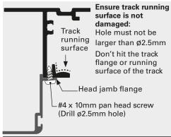
After installation but before lining, clean the full length of the inside running surface of the track with a soft rag, then TAPE UP THE TRACK to ensure no dust or debris enter the track during building works.
