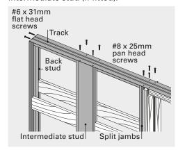
Make sure that the track holes line up with the split jamb and intermediate stud screw tubes.
