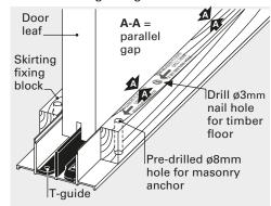
Concrete floor: Ø8 x 90mm masonry anchor Timber floor: Ø3.15 x 75mm nail (not supplied)
