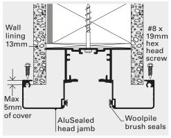
AluSealed head jambs longer than 1m require an extra screw to hold the centre of the jamb to the bottom of the track as shown below.
