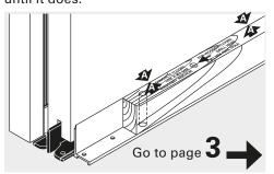
7. The door should now slide smoothly and fit into the recess in the closing jamb, leaving parallel gaps on either side between the door leaf and the closing jamb.
