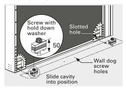
Tighten the screw bolts until the underside of the head is just touching the hold down washer.
